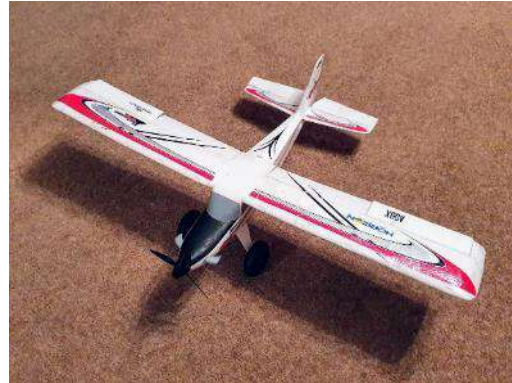
Above right: After a bit of hot water, glue and laminating film to fix the leading edge.
