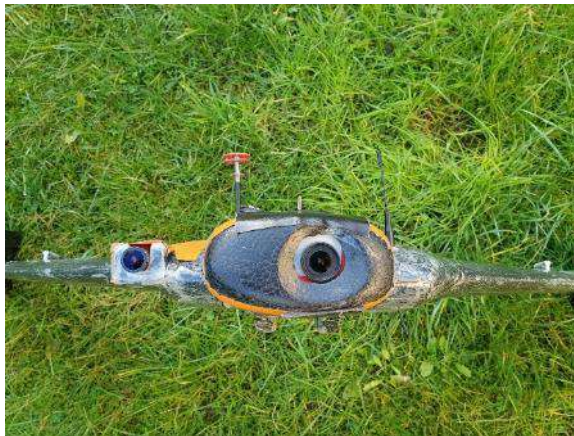
Above left: FPV camera on left, HD recording camera in nose
