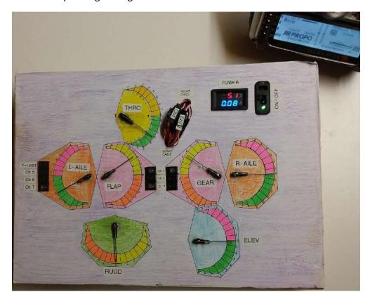
This allows the L-aileron, Flap, and Gear servos to be controlled by any of the channels 5-6 or 7, on the transmitter or even coupled up Y fashion to any at the controls.
