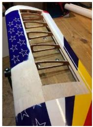
The balsa sides fitted back once steamed over my shed kettle, a good excuse for a cuppa. stick it all back together and clamp up. The building board is essential to ensure a straight line, no one likes flying a banana round the sky. It quickly starts to look like a plane again once you stick some covering over the balsa.
