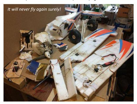
This time it had caused a fair amount of damage; two of the servos were damaged, broken prop and spinner, undercarriage housing, and motor mounting plate. The flaps had disintegrated, but as I never used them anyway, I ended up gluing them solid into the wing. I've never been much into jigsaws, so it was hard to piece it all together. I thought I had picked up every bit of foam from the field, but my annoyance that I'd missed a couple of bits some no smaller than a 1p piece was extreme.
