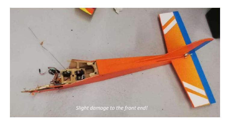
As you can see - not pretty, but the tail still looked good ...... On inspection the failure was caused by both wing bolts shearing at the bolt head.
