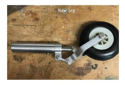
After lots more epoxy was expended gluing the nose leg mount back in and recreating pulverised gear door hinges, it was time to fix the landing light – which had melted itself much earlier in this sorry story. I must be bonkers but I acquired a switching unit to allow the nosewheel light to energise on gear down – the original was on full time...
