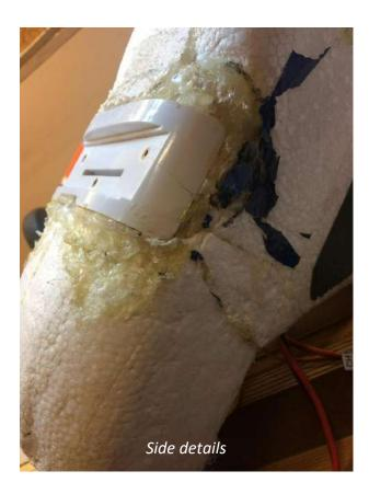
Lining up the fuselage was difficult even after pouring boiling water over the distorted bits. Hence my floats will not fix on without a lot of metal bending if ever.
