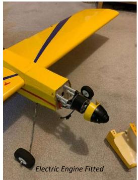
It's the motor numbers that get me! But I think I have finally worked it out. My 650kv motor does 650 rpm per volt. So on 3S which is 12v nominal, it will do 7800 rpm at full throttle which is a bit less than most 4 stroke engines. So it needs a big prop.
