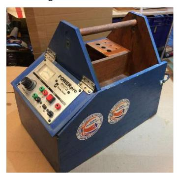
Field box for glow IC setups, with power panel fitted. It has not been connected to fuel as the previous owner has only ever used a hand pump, so I don't know if the pump section works.
