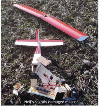
been cautioned by Bill McDiarmid about this possibility only days before! 2 thirds of the front end was smashed to smithereens with a punctured fuel tank, broken engine mount and a broken and bent needle valve.
