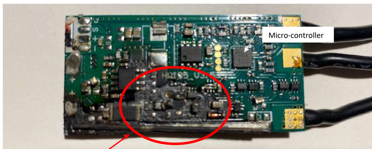
Burnt MOSFETs, heatsink removed
