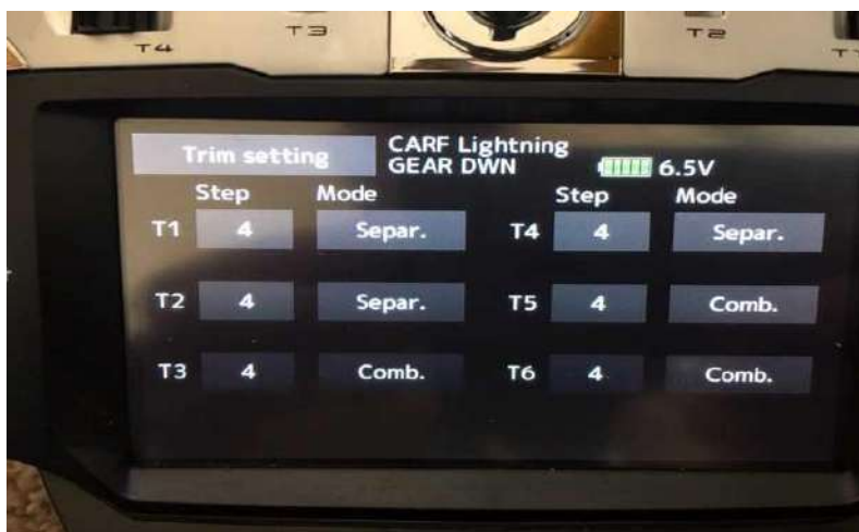
Above: Futaba 18SZ Linkage menu “trim setting” tab showing elevator, aileron and rudder trim separated for adjustment with various flight conditions e.g. flap and landing gear extension etc. (T3 is the throttle trim.. I only use one throttle trim in this installation so it remains in Comb=Combined mode)
