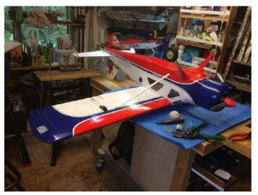
The last thing to do before flying and re-trimming the plane is to double check the rest of the plane for crash damage, and most importantly rebalance the plane both C of G and laterally, as due to the different construction materials and glue it WILL have changed. To do this I hang the plane from the roof, by a screw fitted in the centre of the fuselage where the firewall is, and stand the tail on the bench.
