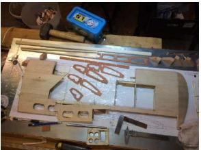
24hrs to dry, which gives me plenty of time to fiddle it into place before clamping it firmly. I have tried using cyno glues but have ended up with twists in the plane as you are turning it over all the time to get the bits in.
