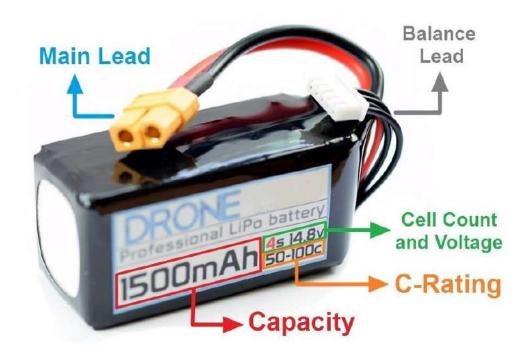
Capacity is expressed on the battery in the form of milliamp hours (mAh). The higher the mAh the longer your electric aeroplane can stay in the air before you have to land and recharge. Of course the larger the capacity the heavier and bigger the battery so ensure that you check the centre of gravity hasn't shifted if you get a bigger battery.
