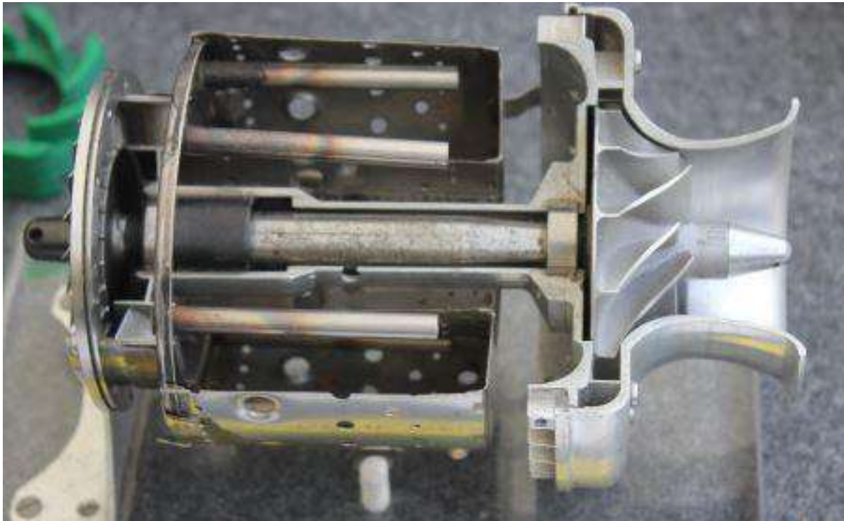
The Jesus Artes KJ66 Engine sectioned.
