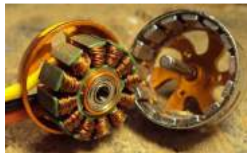
Figure 1: Note the 14 magnets and 12 poles
